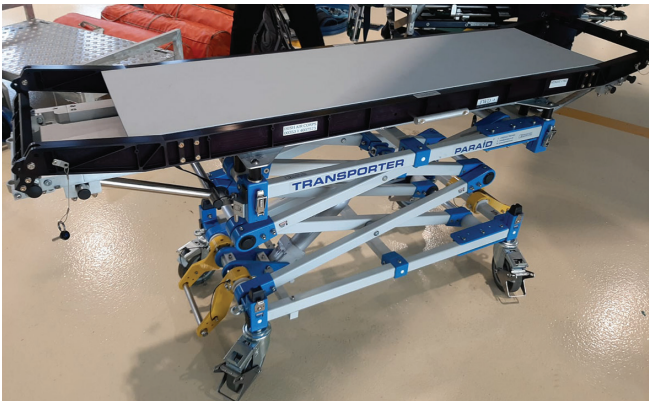
“Interface Plate” (black) for CASA CN 235 Lifeport operations (stored in No 1 Ops Wing storage)
