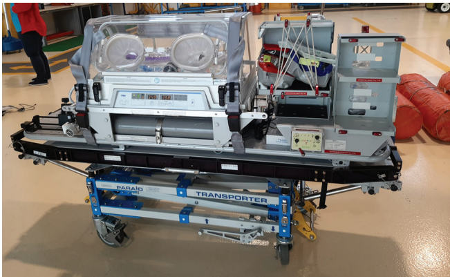
“Interface Plate” (black) for CASA CN 235 Lifeport operations (stored in No 1 Ops Wing storage)
